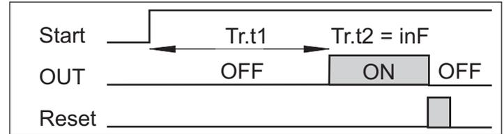
Delayed start at power up with a delay time and a “end of cycle” time
