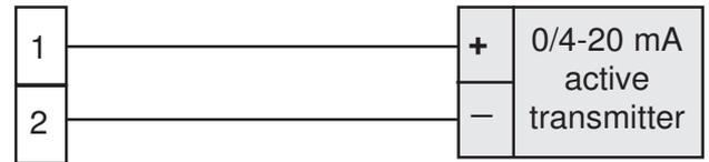
**Fig. 6 0/4-20 mA input wiring for active transmitter**
