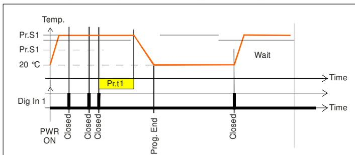
When a new panel is detected before the end of the first soak time, the program restarts and the set point remain
